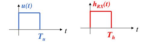
• We can evaluate K for each couple  $(T_u, T_h)$  finding the optimum filter for each pulse, showing that the best filter is not in general the matched filter  $(T_u = T_h)$ .
