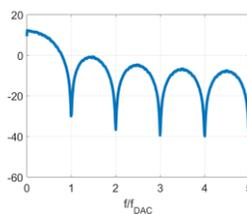
Sample & hold + filter can be compensated for by DSP
