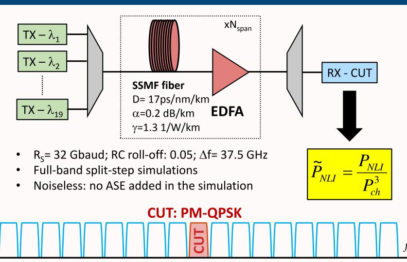
INT: PM-QPSK or PM-16QAM or PM-Gaussian
