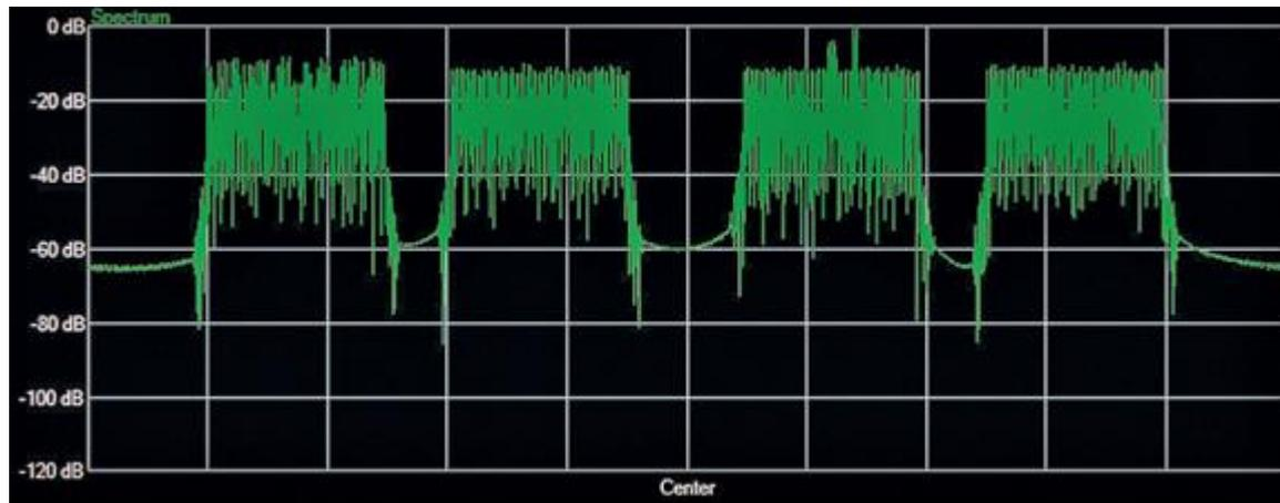
Fig 3. The spectrum of the LTE-Advanced configuration includes four non-contiguous 20-MHz carriers <http://electronicdesign.com/4g/wireless-companies-follow-roadmap-past-4g-and-5g>
