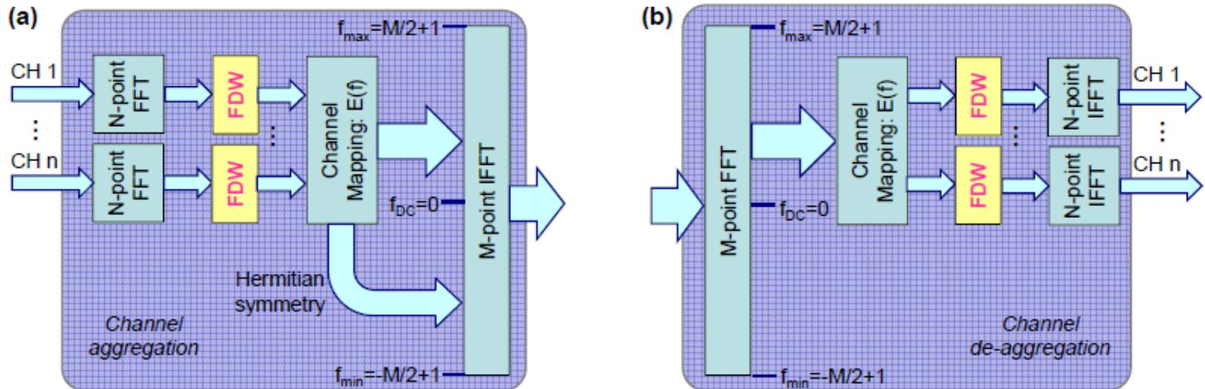
**Fig. 2:** Schematic of the DSP blocks for FFT/IFFT-based channel aggregation (a) and de-aggregation (b), both with the use of frequency-domain windowing (FDW) to reduce the DSP processing latency.
