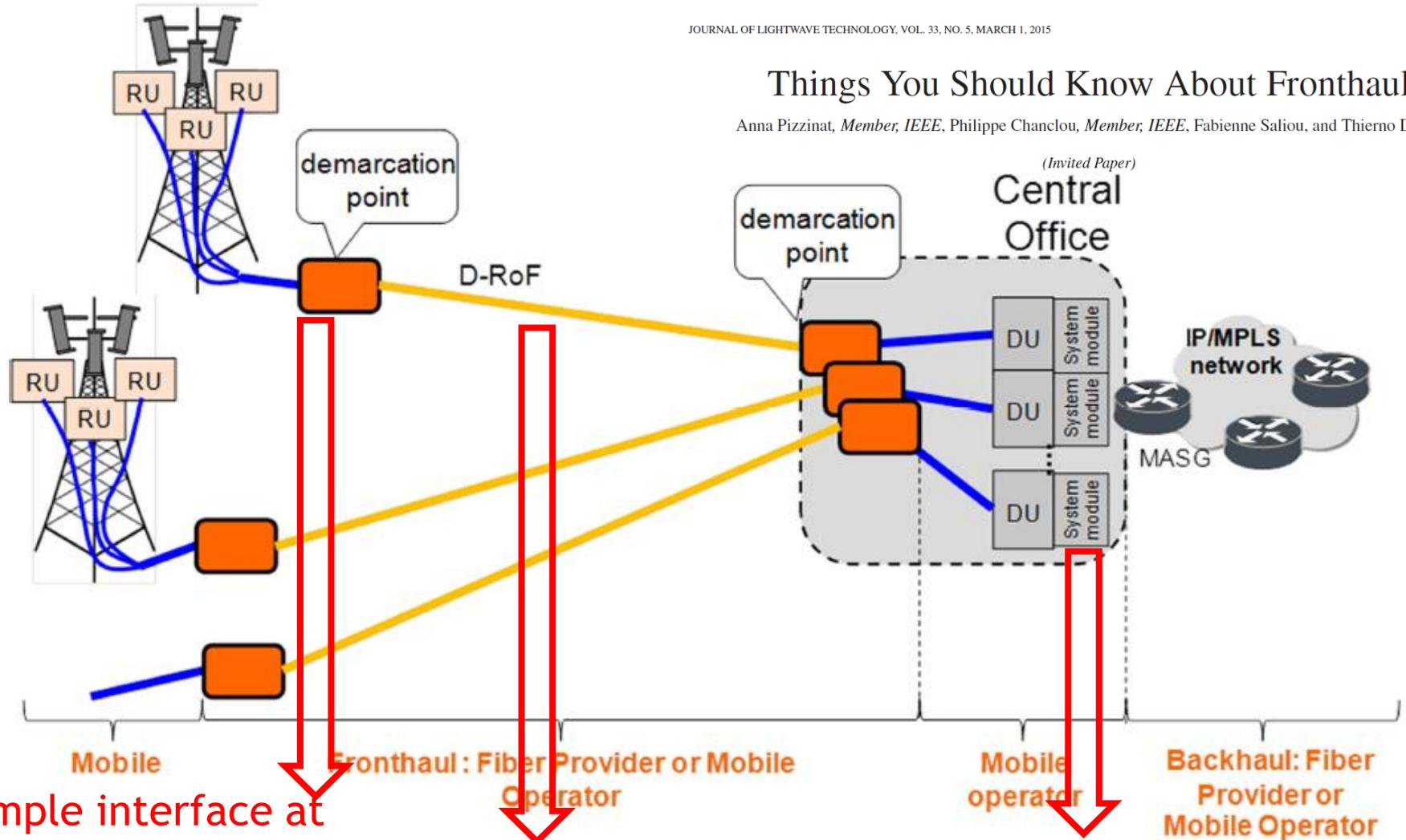
Simple interface at antenna site (RRH: Remote Radio Head)
