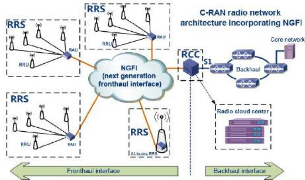
Figure 2-1: C-RAN Radio Network Architecture Based on NGFI
