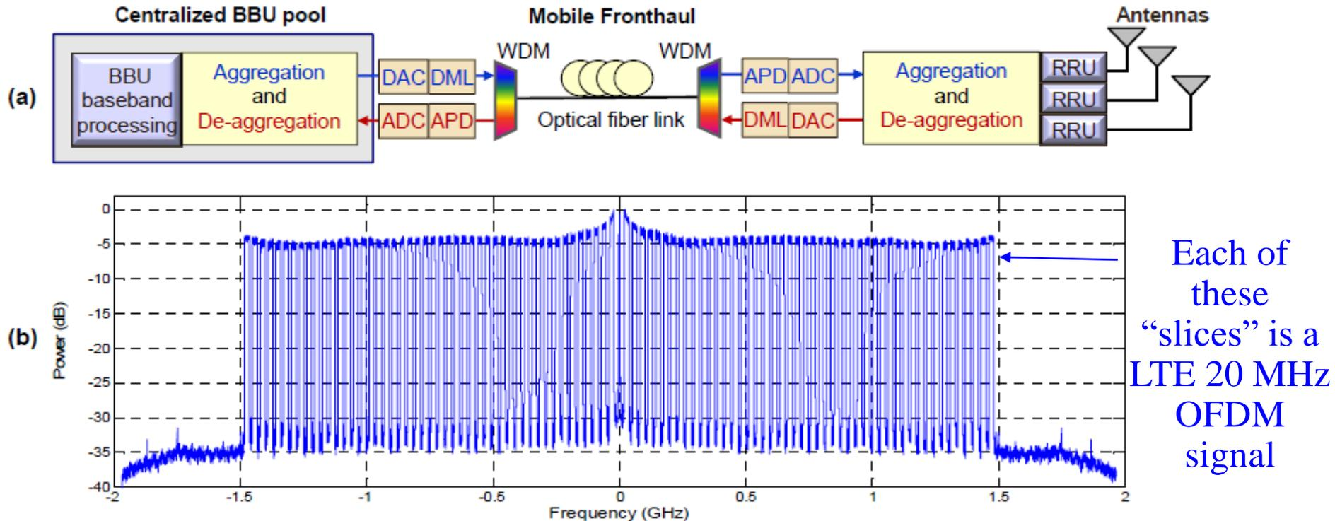
**Fig. 1:** (a) Schematic of the mobile fronthaul architecture with DSP-based channel aggregation and de-aggregation in the frequency domain; (b) Experimentally measured spectrum of 48 20-MHz LTE signals (and their images due to Hermitian symmetry) that are aggregated using seamless channel mapping and transmitted over 5-km SSMF with -6 dBm received signal power. The signal center wavelength is 1550 nm. DML: directly modulated laser; APD: avalanche photodiode.
