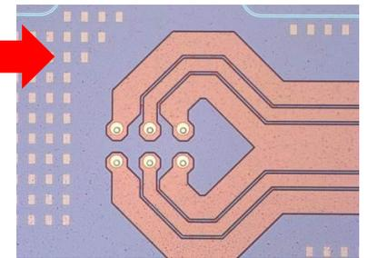
*RF electrodes with pads for bump interconnections*
