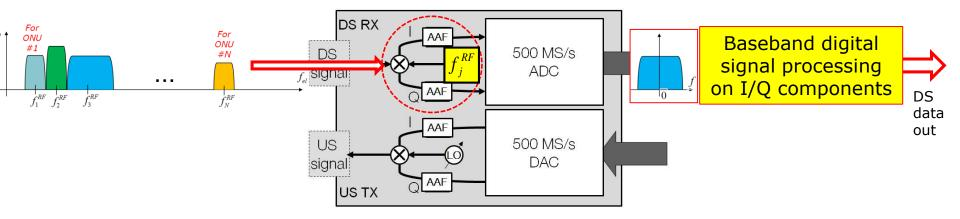
For instance, targeting 1 Gbps per ONU, and using 16-QAM, the required baseband processing can be done using DAC and ADC working in the 500 Msample/s range
