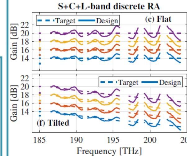
(c),(f): Predicted and target flat and tilted (on-off) gain profiles with respect to frequency
