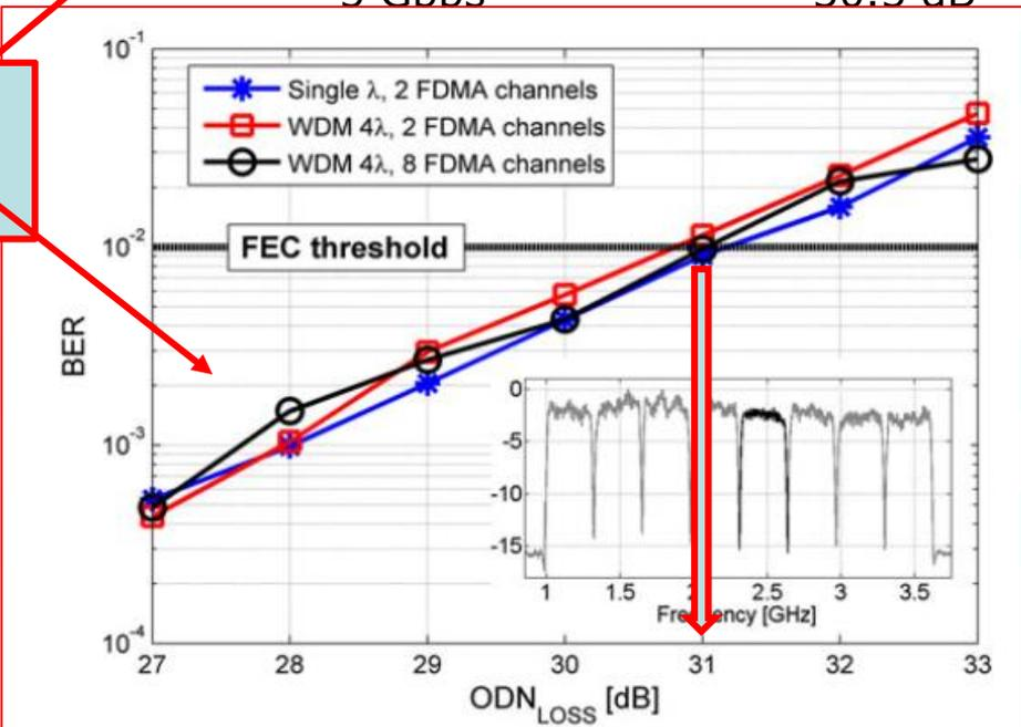
Fig. 2. Performance of the upstream transmission in terms of BER vs ODN loss with two active ONUs (32 emulated channels per wavelength using optical noise loading). It is evident that the simplified setup totally emulates the meaningful interferences.
