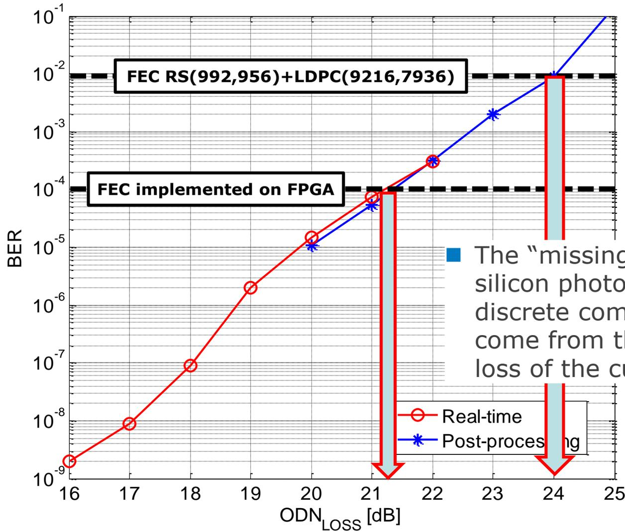
■ The “missing” 7 dB between the silicon photonic setup and the discrete components one mostly come from the higher insertion loss of the current prototype
