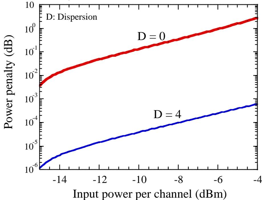
Curves are derived using Gaussian approximation.
