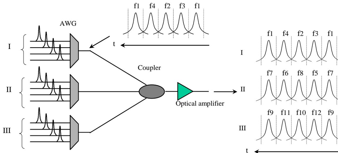
Channels are equally spaced in frequency domain.
